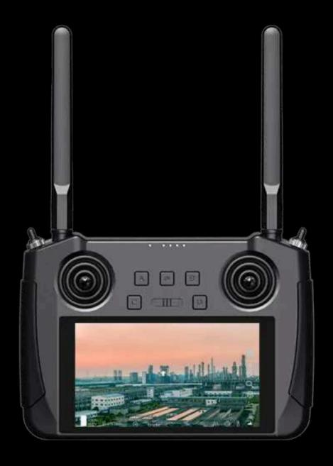
MK15E is a long-range Android smart controller with dual 1080p FPV, based on the full high-definition image transmission technology developed by SIYI Technology.
